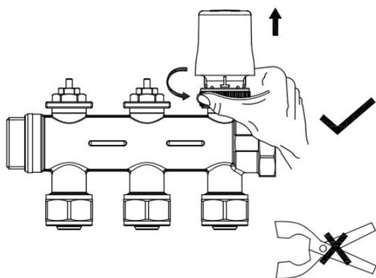
Rotate the nut anticlockwise, push up along the spool spring until remove the actuator.
